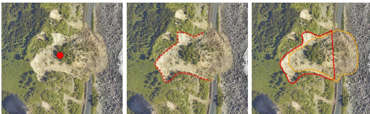
Figure 8 Examples of how landslides are depicted in GIS (A) Point within the landslide body; (B) Line around the head scarp of the landslide; (C) Polygons delineating the failure zone (red solid line) and the debris runout zone (orange dashed line)
