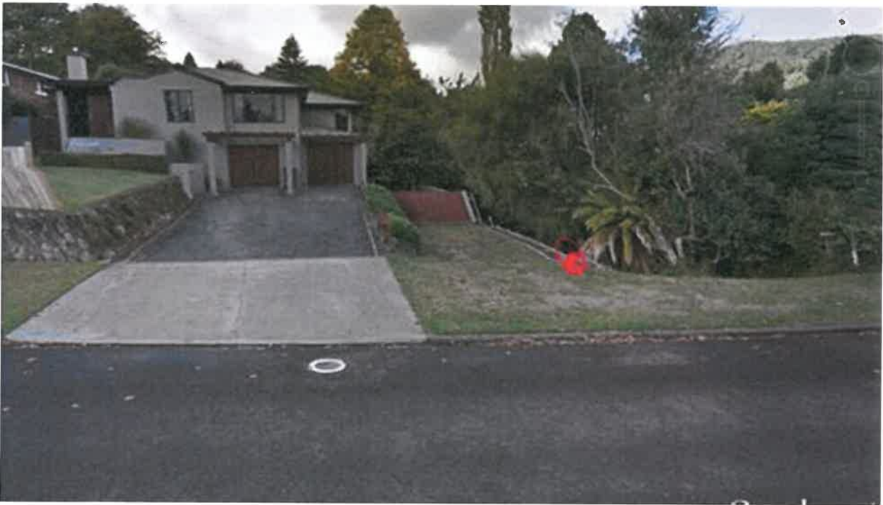
Figure 8-4: Red dot marking location of recorded flood level upstream of Selwyn Road culvert inlet. Flood mark recorded at 305.172 m above Moturiki datum.
