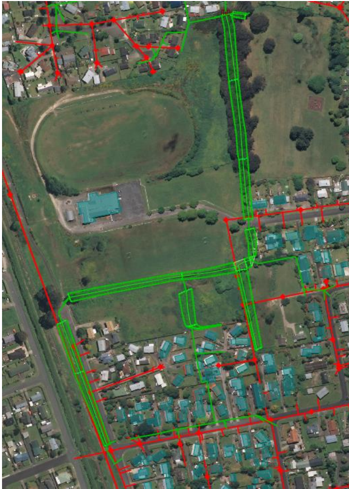
Figure 3: Stormwater network (green) and wastewater network (red) in the Frank Street/Ian Street area to trash screen
