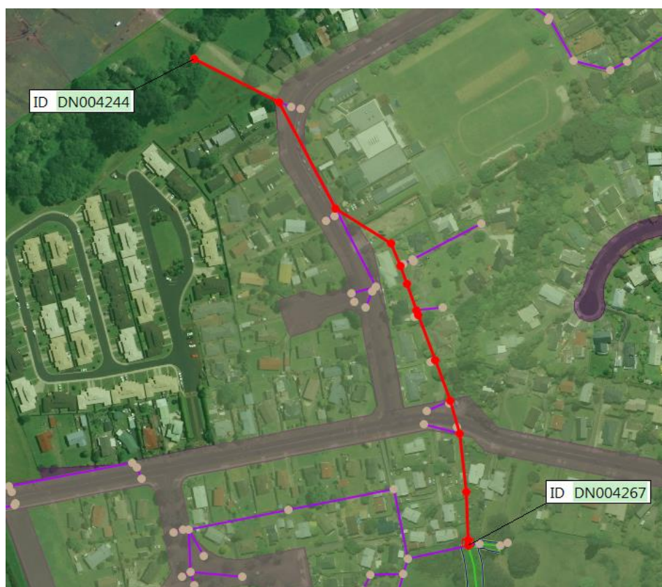
Figure 23: Plan view of the long section from trash screen (DN004267) to the outfall to the stream (DN004244)
