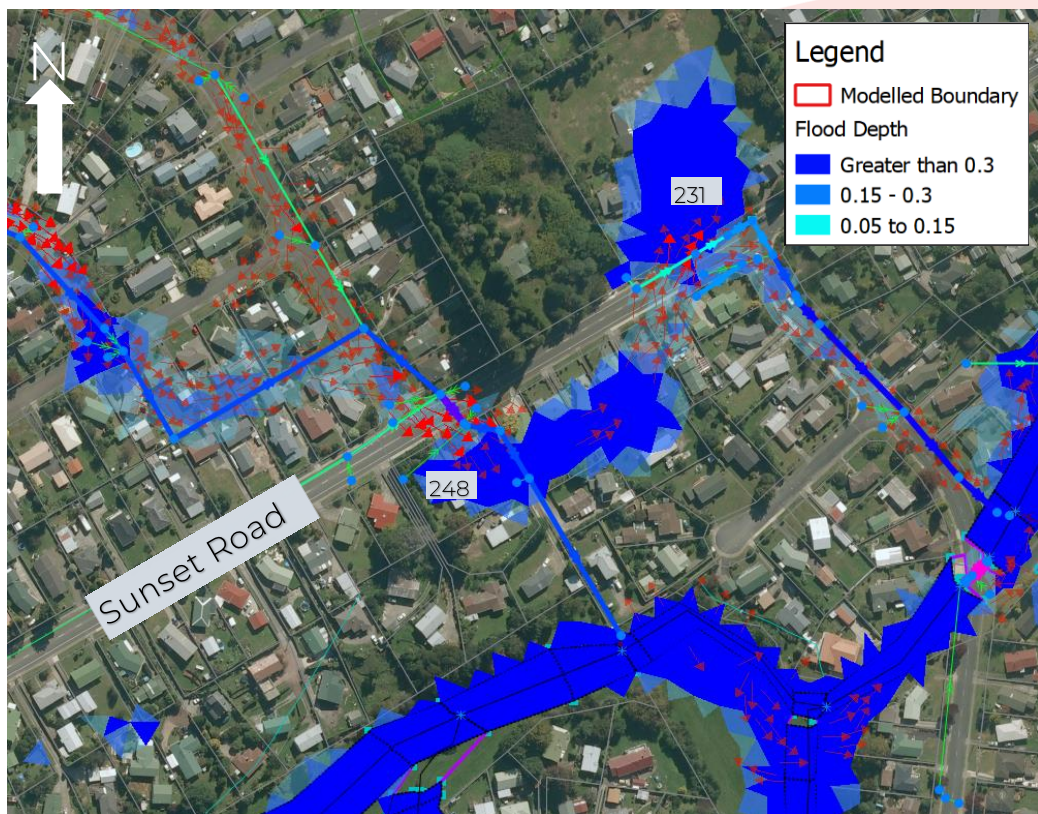
Figure 5-4: 231 and 240-248 Sunset Road Flooding
