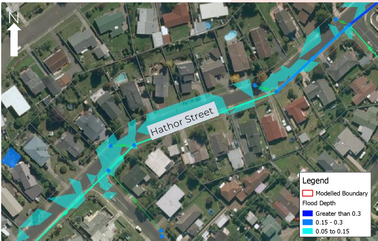
Figure 4-7: Example of road flooding
