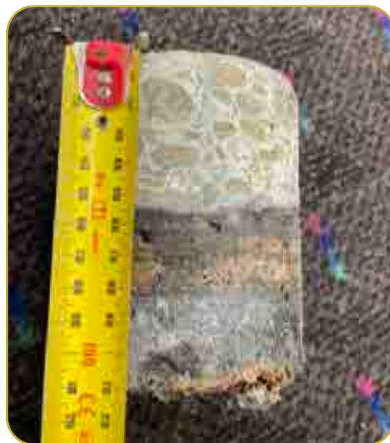
Figure 7 Concrete core showing effects of geothermal corrosion (Photo: Ash Bowtell)
