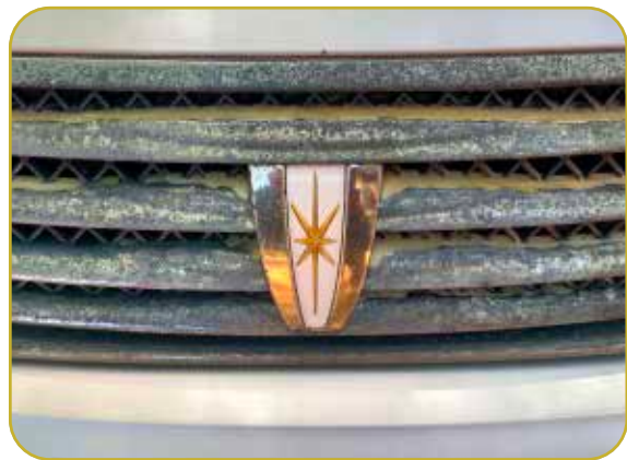
Figure 9 Accelerated corrosion on a Rotorua vehicle (Photo: Kim Smith, January 2024).
