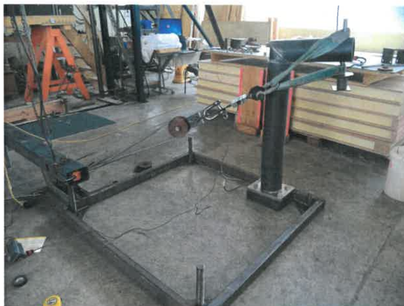
Figure 32. Foundation attachment proof test setup
