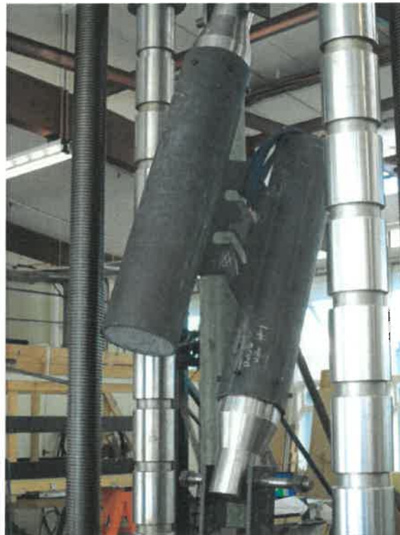
Figure 29. Standard chevron proof test setup
