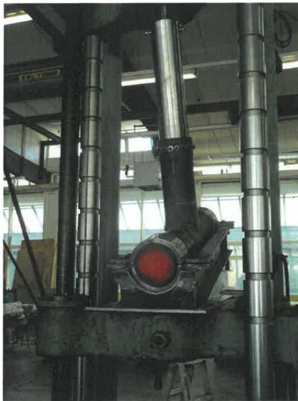
Figure 31. Tube to tube connection proof test setup
