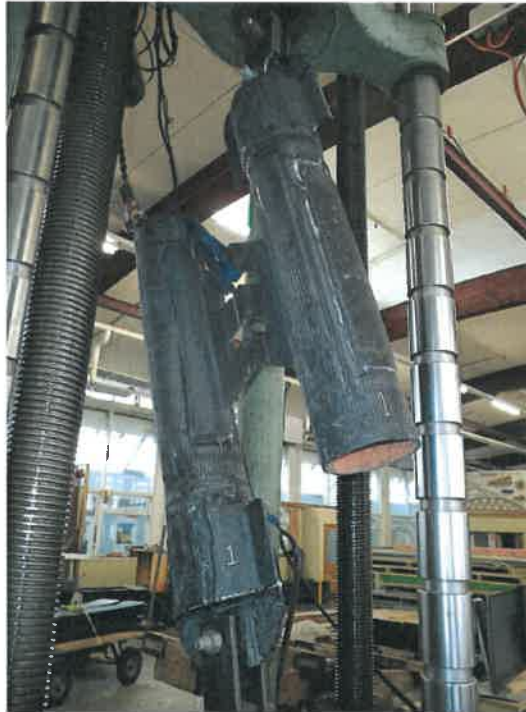
Figure 30. Through chevron proof test setup
