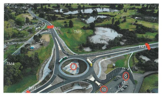
Traffic is to be halted at locations TM1, TM2, TM3 and TM4 when ML is in position and ready for install at Location 8. Once each helix is bolted into place and ML is back to Location 8 traffic can be released again.
